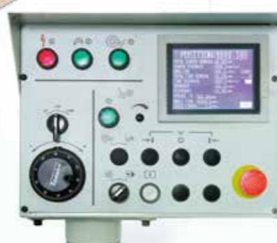
Automatic infeed models (NC) are equipped with a PLC touch screen control with easy to learn conversational software.
