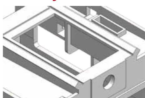
A double inverted "V" slideway with optimum spacing for the regulating wheel assembly provides smooth movement and stable grinding operation.
