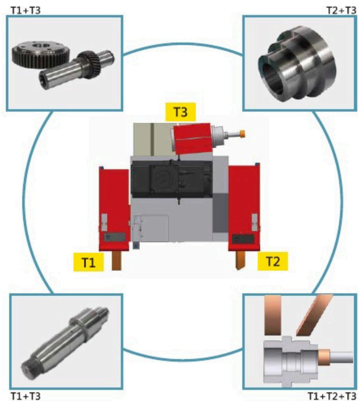
Process ID φ6~φ150mm (Wheel diameter max.60mm) Max. travel 600mm (Exclude chuck)
