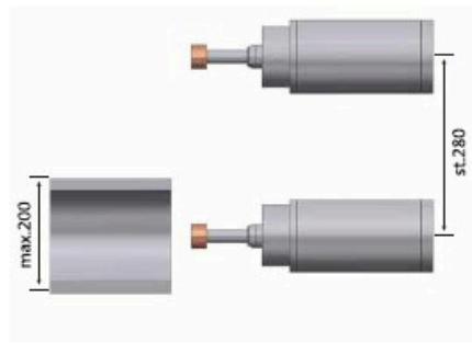
Process ID φ6~φ150mm (Wheel diameter max.60mm) Max. travel 600mm (Exclude chuck)
